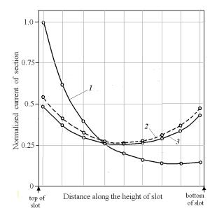
Figure 7. Distribution of current in the sections of winding at the frequency 400 Hz (1 is the mode of compression; 2 are the inner sections, mode of excitation; 3 are outer sections, mode of excitation). The basic current is equal to 1 A
