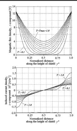
Figure 11. Results of simulation for the flux switch in across the conducting plate likely to Shield 1
