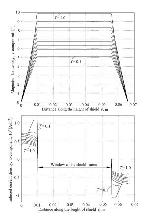
Figure 12. Results of simulation for the conducting frame likely to Shield 2 at the fast switch in of the flux in the window of frame
