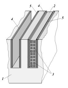
Figure 2. Using of the Shield 1 in the model (*1* is the ferromagnetic core, 2 is the winding package, 3 is the sections of winding, 4 is the copper plate at left side of slot, 5 is the copper plate at the right side of slot)
