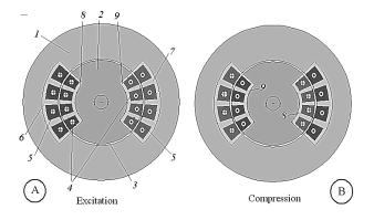
Figure 8. The cross section of the compression generator at two positions of rotor: A – for the excitation of the initial magnetic field, B – for the stage of the flux compression. Designations: 1 is the stator core, 2 is the rotor core, 3 is the air gap, 4 is the rotor winding, 5 is the stator winding, 6 and 7 are the block-keepers of stator winding, 8 and 9 are the blockkeepers of rotor winding
